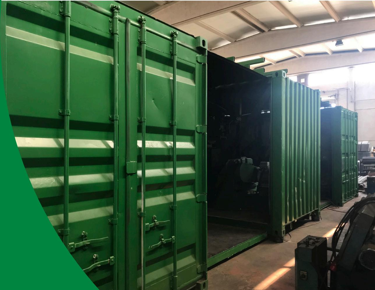
*All 3 ton triple deck Organic Waste Systems are housed in four parallel transport ready containers 40' x 8' (12.2M x 2.4M).*
